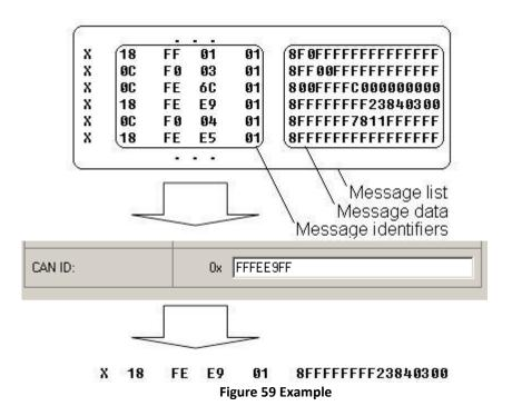
When certain message is filtered, FM5300 checks which data bytes should be sent to server. Document indicates that 5-8 bytes are used in FMS standard.
