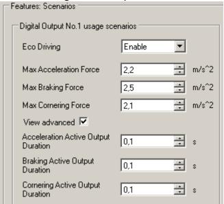
Figure 48 ECO driving configuration parameters
