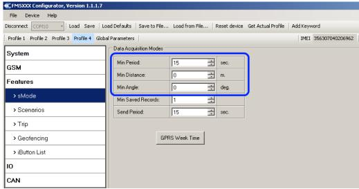
Figure 36 GPS acquisition configuration window
