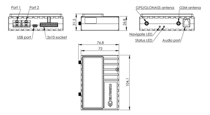
Figure 1 FM5300 view & dimensions in mm (tolerance ±2mm)
