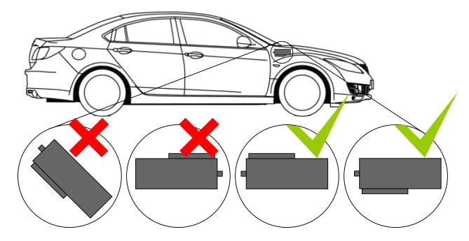
Figure 45 Correct mounting position of the FM5300 in the vehicle
