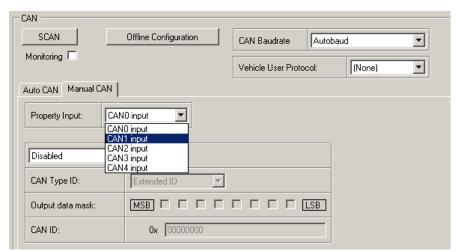
Figure 53 CAN configuration window
