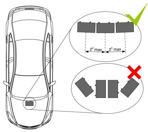
Figure 47 Horizontal position MAX deviation of FM5300 mounting
