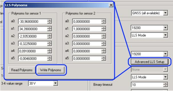
Figure 78 LLS sensor advanced (polynomial) setup
