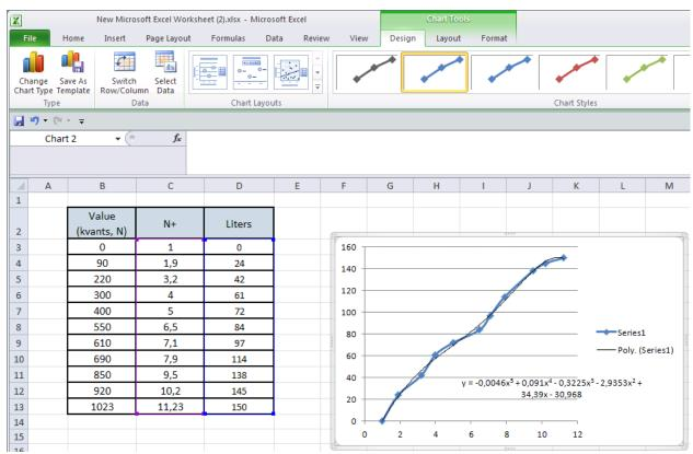
Figure 76 Calculated polynomial line and calculation formula
