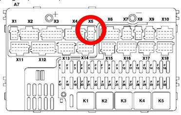
Figure 57 X5 plug on Mercedes Benz
