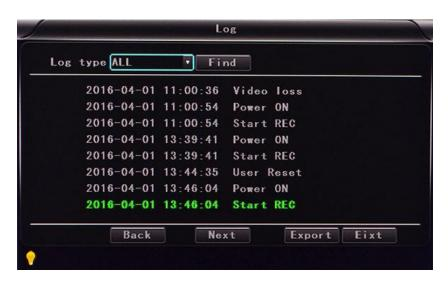
✓ **Log type**: User action log, alarm logging, equipment status log.
