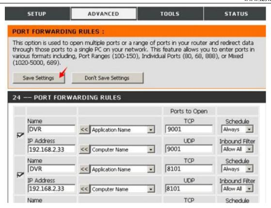
✓ After the port mapping settings, find the "IP Address" in the WAN, the IP Address is your CMS server IP.
