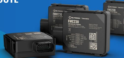
All the great features of the acclaimed FMx1 series devices are now available with IP67 certified casing – as an expansion of waterproof FMx2 series trackers.
