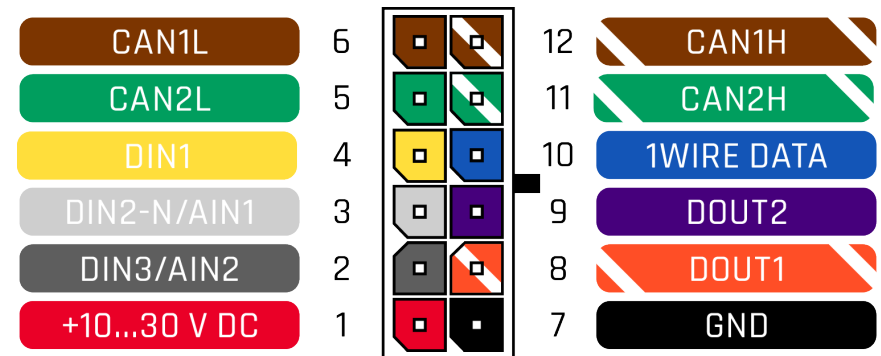
Figure 2 FMB240 2x6 socket pinout
