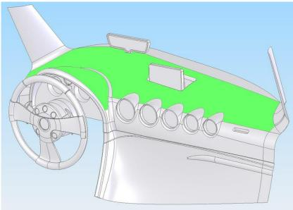
Figure 53 Correct placement of FM1100
