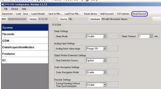
Figure 19 FM11XX Configurator window with FM1100M connected
