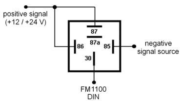
Figure 12 Inverting relay connection
