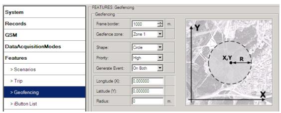
Figure 37 Geofence configuration
