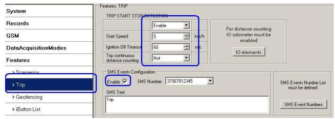
Figure 42 Trip Start/Stop SMS event configuration
