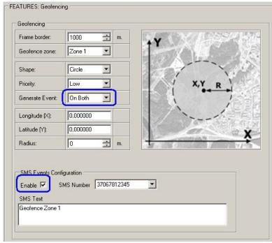
Figure 43 Geofence SMS event configuration
