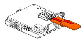
3 Step for FM1100M+2SIM version: Insert SIM cards as shown. Lower slot is for SIM 1, upper slot is for SIM2.
