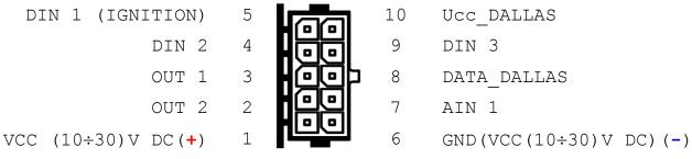
Figure 5 2x5 socket pinout
