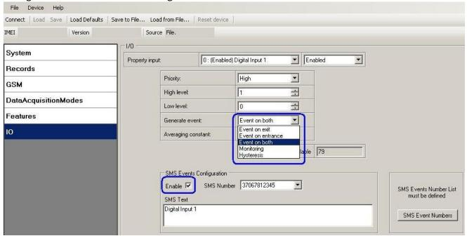
Figure 45 I/O SMS event configuration
