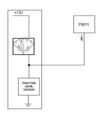
Figure 10 Fuel sensor scheme
