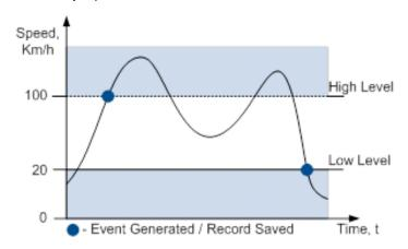
Figure 50 Event generation according hysteresis algorithm
