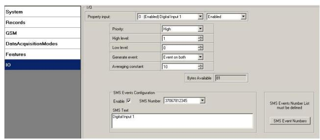
Figure 40 Configured Digital Input 1 SMS event
