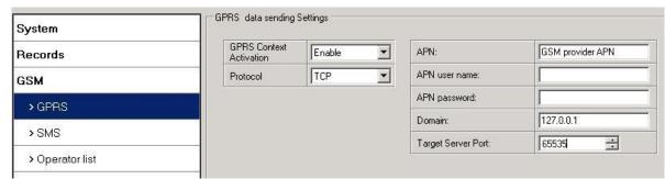
Figure 26 GPRS configuration
