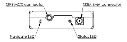
Figure 1 FM1100 view & dimensions (tolerance ±2mm)
