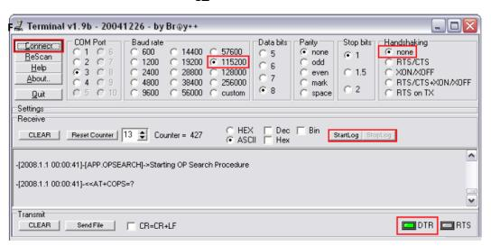
Figure 51 Terminal window for logging
