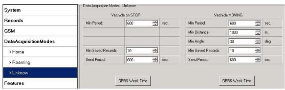
Figure 31 Data Acquisition Mode configuration
