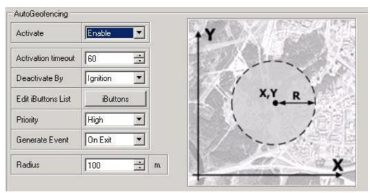
Figure 38 Geofence configuration
