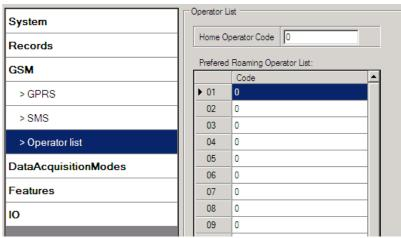
Figure 28 Operator list configuration
