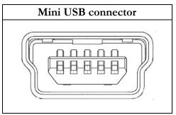
Figure 6 Mini USB type B connector
