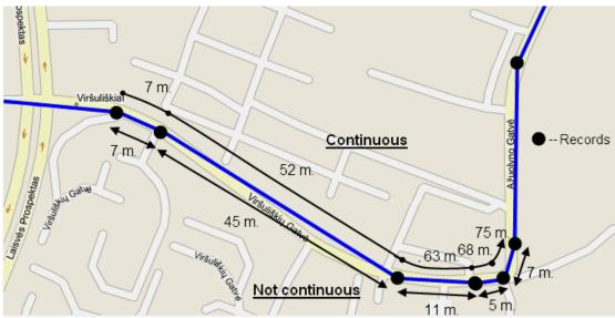
Figure 35 Trip continuous distance counting parameter example
