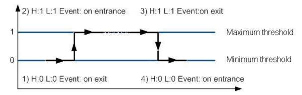
Figure 48 Digital Input event generation example
