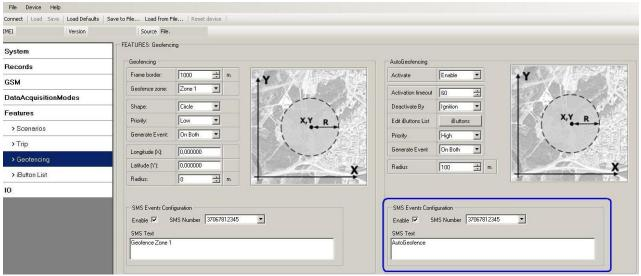
Figure 44 AutoGeofence SMS event configuration
