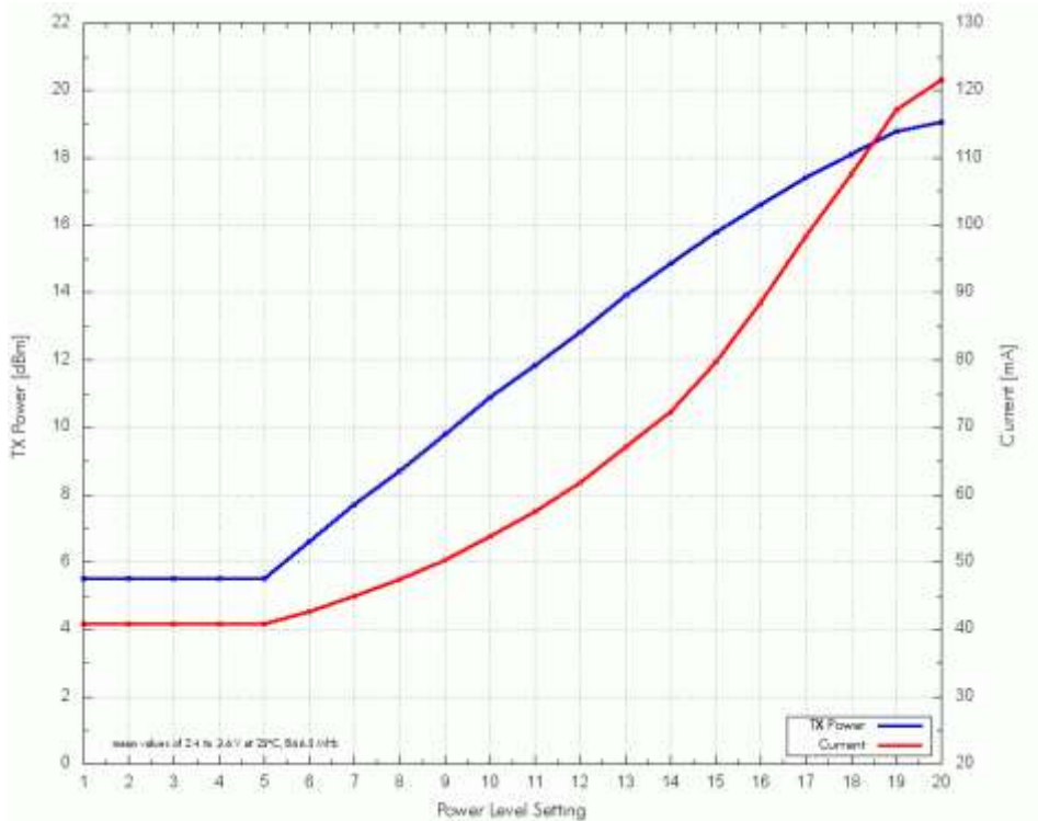
Figure 4-1: RF output power level and current consumption versus power stages from 1 to 20 @ room temperature
