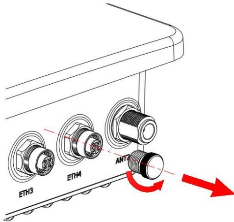
2. Connect an Ethernet cable to any port marked ETH0~ETH4 at the bottom of the enclosure, and rotate it clockwise.
