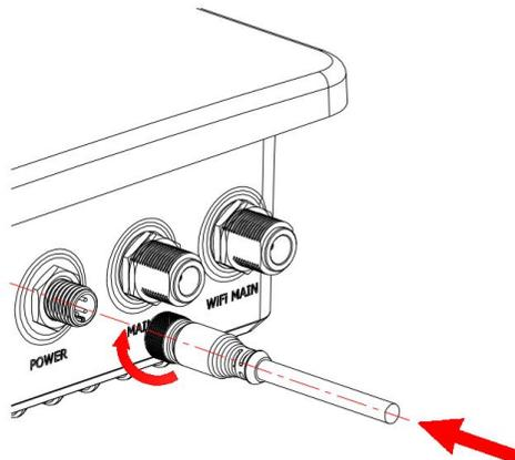
3. Connect the other end of the cable to your specific power supply source.
