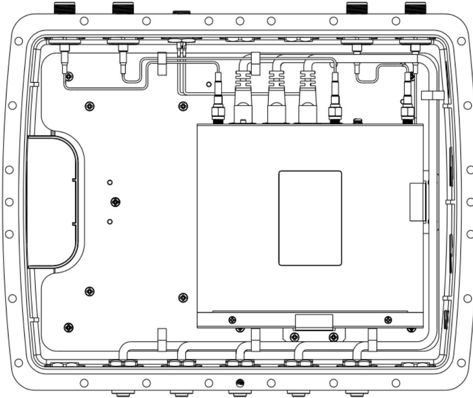
2. Disconnect all cables or wires of the router and take it out.
