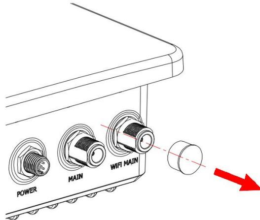
2. Connect the antenna to the corresponding antenna connector by holding onto the metal part of the antenna and rotating it clockwise.
