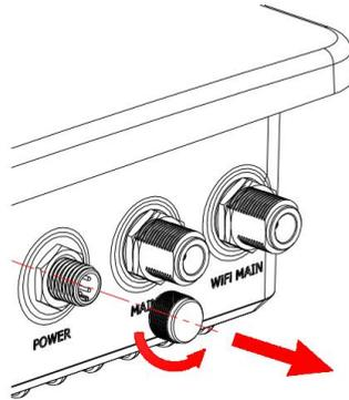
2. Connect a power supply cable to the power port, and rotate it clockwise.
