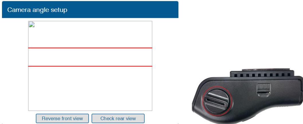
In case of indoor installation or somewhere you cannot see the horizon properly, use same data to "**Camera Height**". Mark the same height on the wall apart about 3 ~ 5 meters from the vehicle.
