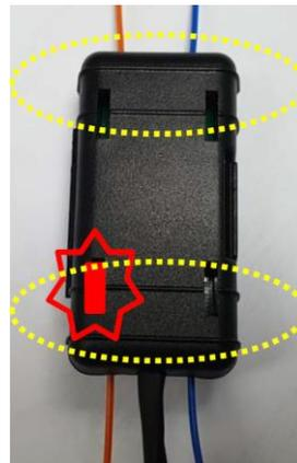
\* After checking on operating of LED lights correctly, tie with a cable tie marked in yellow.
