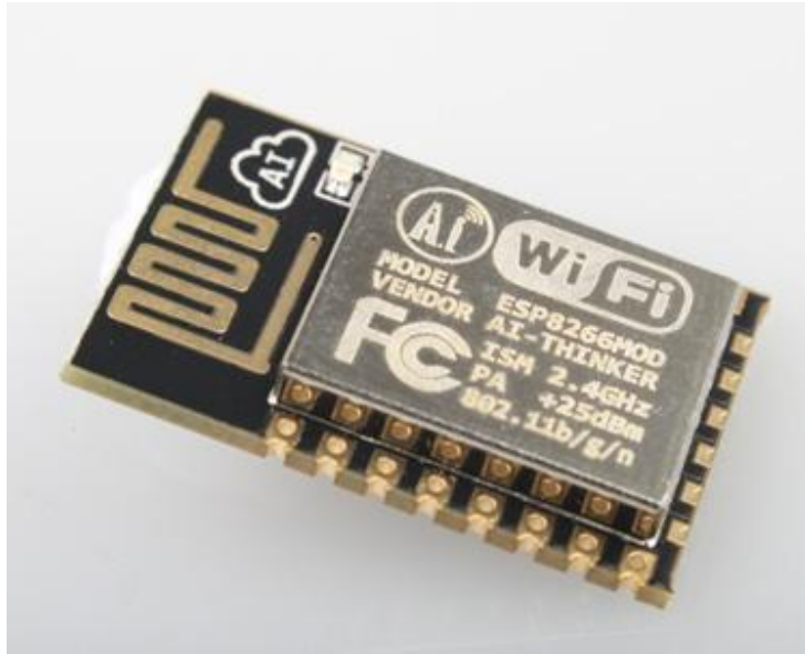
Figure 3 [Module Pin Counts, 22 pin, 16 mm *24 mm *3 mm]
