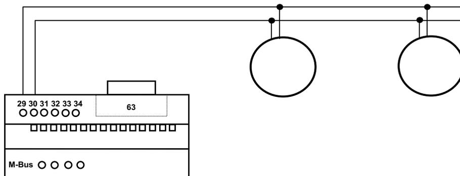
Any cable type may be used as long as the cable is suitable for 42 V / 500 mA. Shielding is not necessary and not recommended since the capacity of the cable should be minimized.
