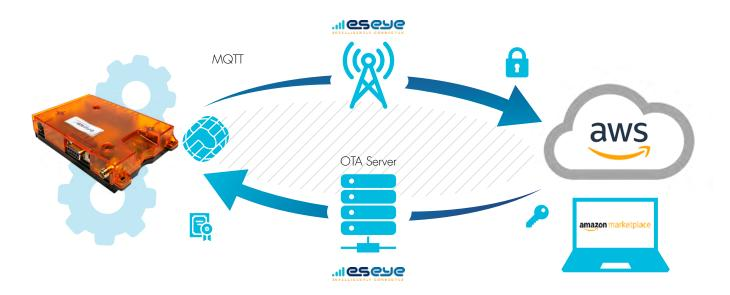
The solution delivers pre-installed firmware in the IoT terminal which intelligently manages security, connectivity and credentials between the device and the cloud, ensuring a consistent global 'out of the box' experience. The device behaviour simplifies IoT deployment and automates global, secure connectivity into AWS IoT Core.
