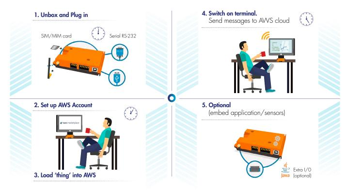
The PLS62 Terminal uses either RS232 or USB to connect to the host device. This is ideal for use cases where the host device is able to send AT commands. Further connectivity is provided using the expansion connector offering SPI, I2C, GPIO, an additional RS232 interface and 5v power supply. For
