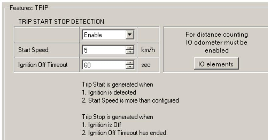
Figure 23 FM53 Features->Trip Configuration
