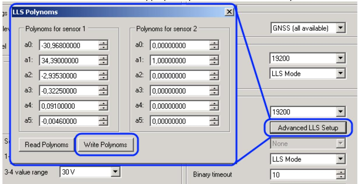
**Figure 78 LLS sensor advanced (polynomial) setup**
