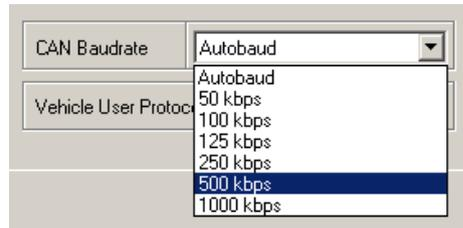
Figure 54 CAN baud rate configuration window
