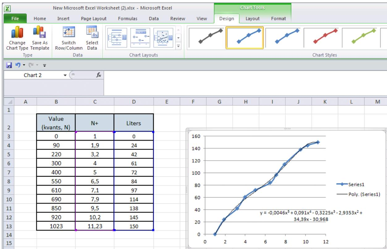
Figure 76 Calculated polynomial line and calculation formula
