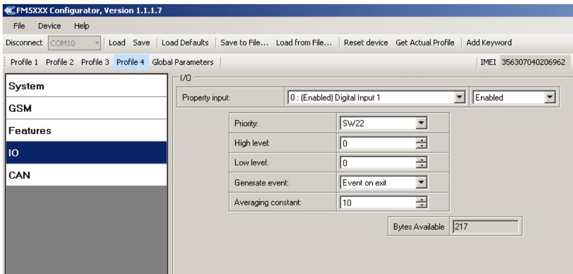
Figure 34 Switch to profile on event (1)
