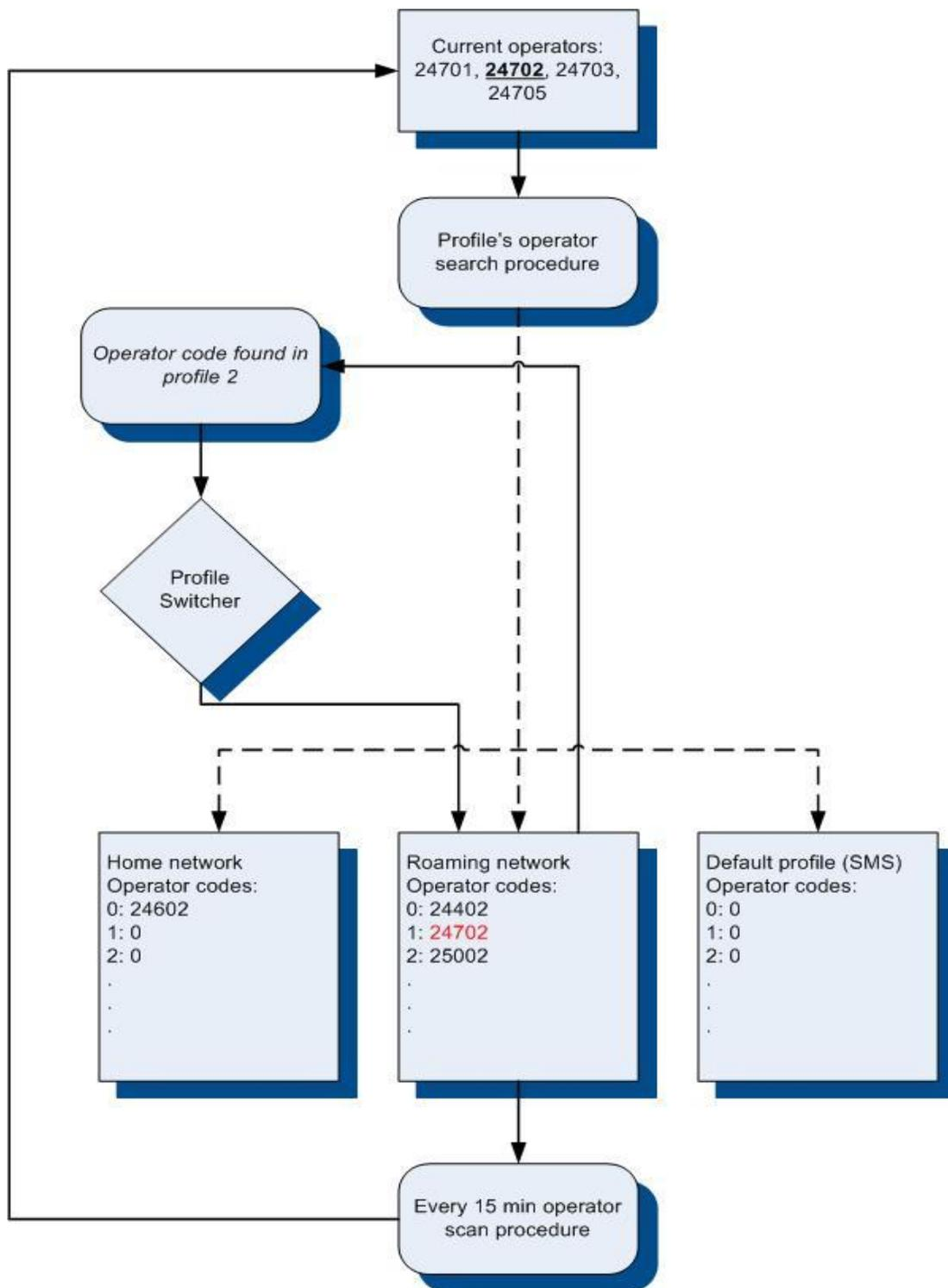
Figure 32 GSM Operator code profile switching (...)
