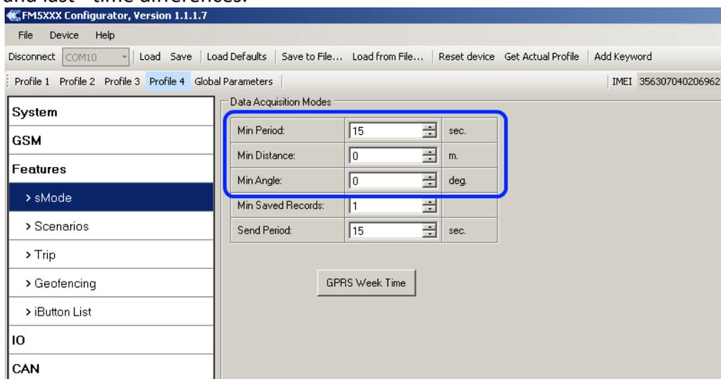
Figure 36 GPS acquisition configuration window
