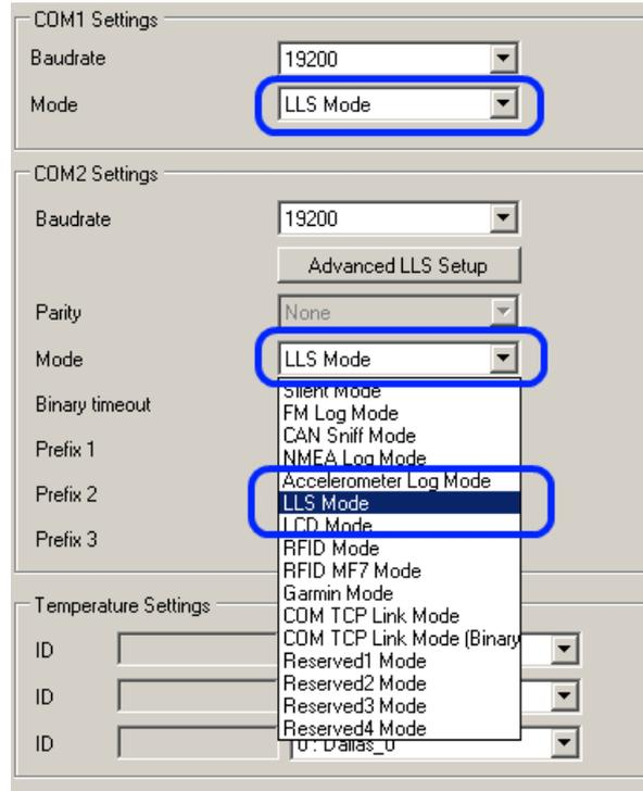
**Figure 77 LLS mode settings in Global parameters**
