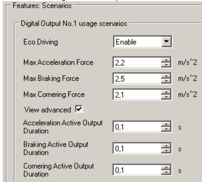
Figure 48 ECO driving configuration parameters
