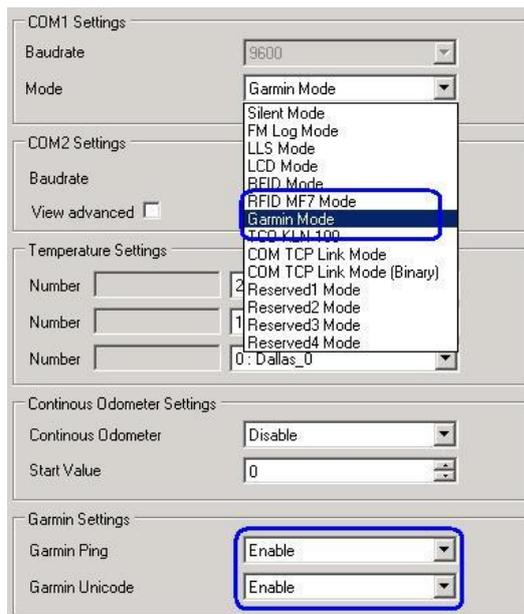
Figure 69 Configuration of Garmin in Global parameter settings
