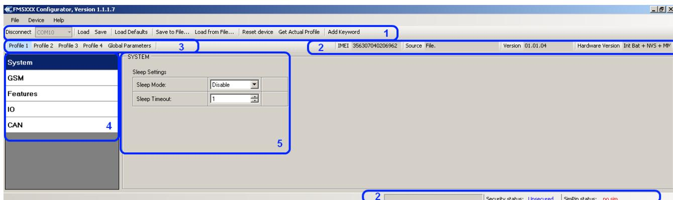
Figure 12 FM5300 Configurator window structure
