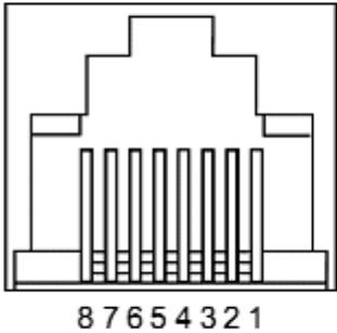
Figure 68 RJ45 Pinouts
