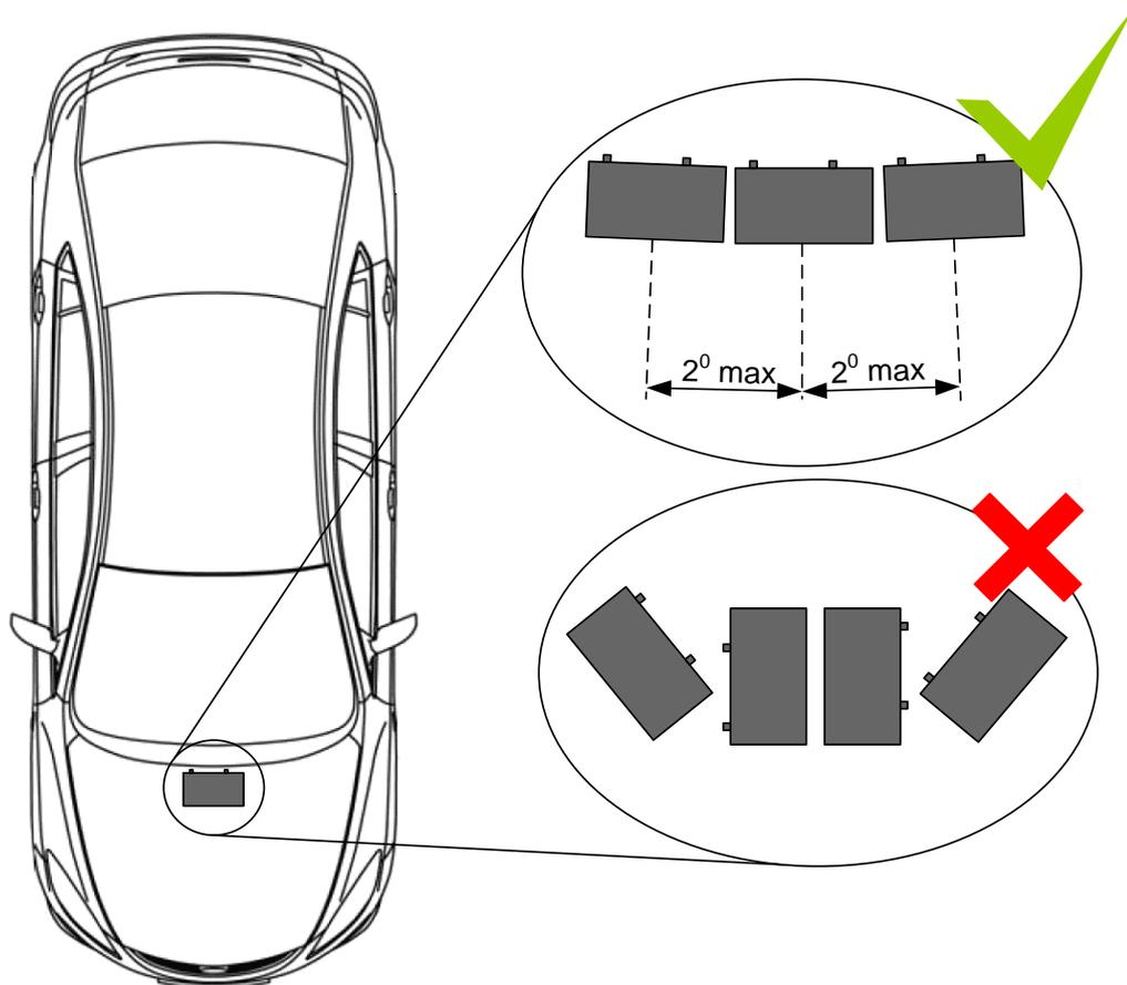
Figure 47 Horizontal position MAX deviation of FM5300 mounting
