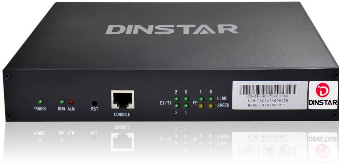
Figure 1-2-2 MTG200 Front View
