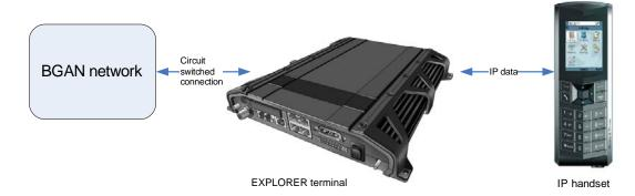
When connected to the terminal the IP handset provides a dedicated BGAN menu with a subset of the terminal configuration options.
