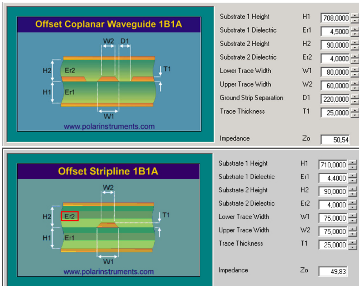
Figure 19: Embedded Stripline line arrangement
