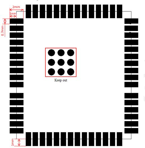
Figure 6-2 PCB foot print of W30 (top view)
