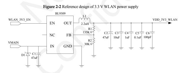
In Figure 2-2, use TVS at D1 to enhance the performance of the module during a burst. SMF5.0AG is recommended. A large bypass tantalum capacitor (47  $\mu$ F) is expected at C2 to reduce voltage drops during bursts together with C3 (10  $\mu$ F ceramics capacitor). In addition, add 0.1  $\mu$ F and 100 pF filter capacitors to enhance the stability of the power supply.
