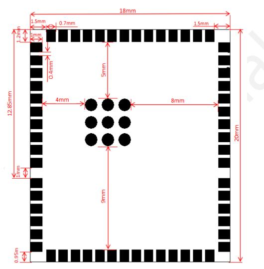
Figure 6-1 W30 dimensions(top view)
