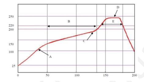
Figure 8-1 SMT furnace temperature curve
