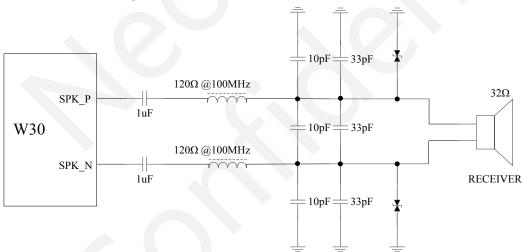
Figure 2-17 Reference design of the receiver circuit
