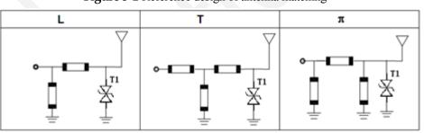
Figure 3-1 Reference design of antenna matching
