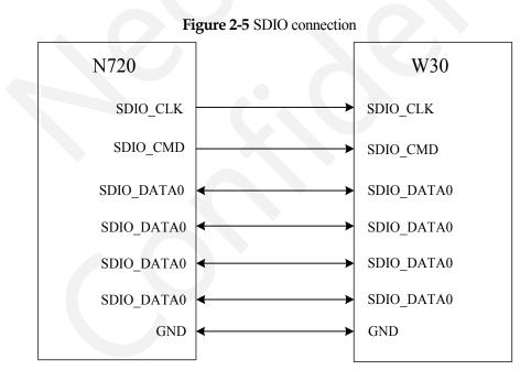
CLK, CMD, DATA0, DATA1, DATA2 and DATA3 are high-speed signal lines. Limit their characteristic impedance to  $50\Omega$  and do not allow them to cross any other traces. Ensure length matching for CMD, DATA0, DATA1, DATA2 and DATA3 traces. CLK trace should be grounded separately.
