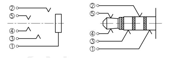
Please note if the headphone is CTIA or OMTP. The connections of ① and ② are reverse for the two type of headphones. The JD1 pin (⑤ in the above figure) is unconnected if the headphone is not plugged. After the headphone is plugged, this pin is connected to GND through the left channel (8/16/32  $\Omega$ ) loudspeaker of the headphone.
