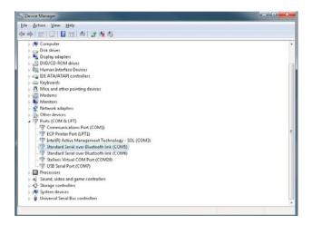
*Note:* Windows assigns two COM ports after completion of the XDL ROVER 2 pairing process. Always select the first COM port that was assigned. For example, if COM 5 and COM 6 were assigned after the pairing process, COM 5 is the correct port to use for connecting to the XDL ROVER 2.
