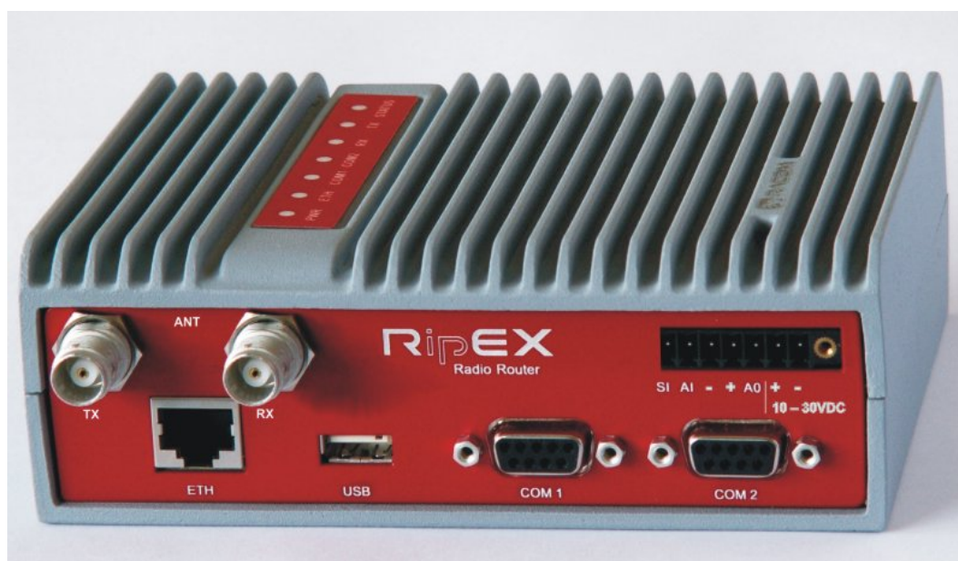
Fig. 3.5: Separated Rx and TX antennas
