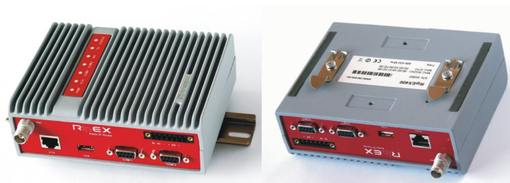
Fig. 5.1: Flat lengthwise mounting to DIN rail – recommended
