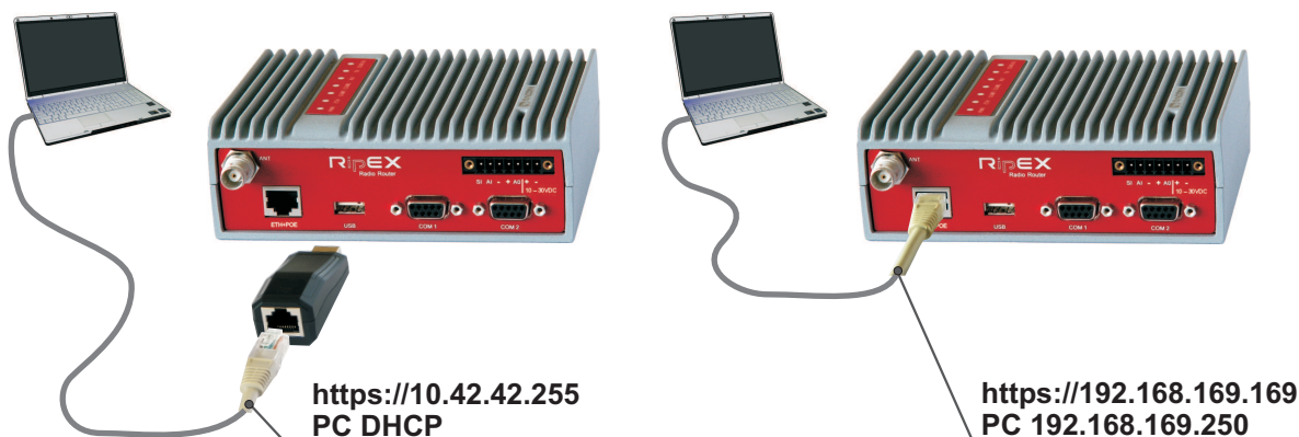
Fig. 4.2: Connecting to a PC over ETH and over ETH/USB adapter
