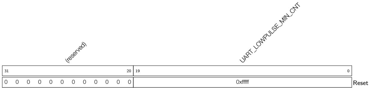
**UART\_LOWPULSE\_MIN\_CNT** This register stores the value of the minimum duration time of the low level pulse. It is used in baud rate detection. (RO)
