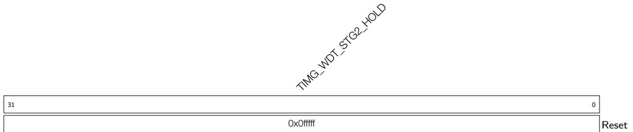
**TIMG\_WDT\_STG2\_HOLD** Stage 2 timeout value, in MWDT clock cycles. (R/W)
