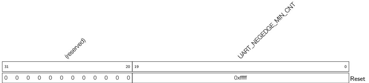
**UART\_NEGEDGE\_MIN\_CNT** This register stores the minimal input clock count between two negative edges. It is used in baud rate detection. (RO)
