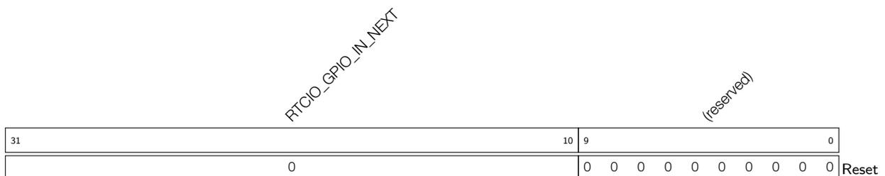
**RTCIO\_GPIO\_IN\_NEXT** GPIO0 ~ 21 input value. Bit10 corresponds to GPIO0, bit11 corresponds to GPIO1, etc. Each bit represents a pad input value, 1 for high level, and 0 for low level. (RO)
