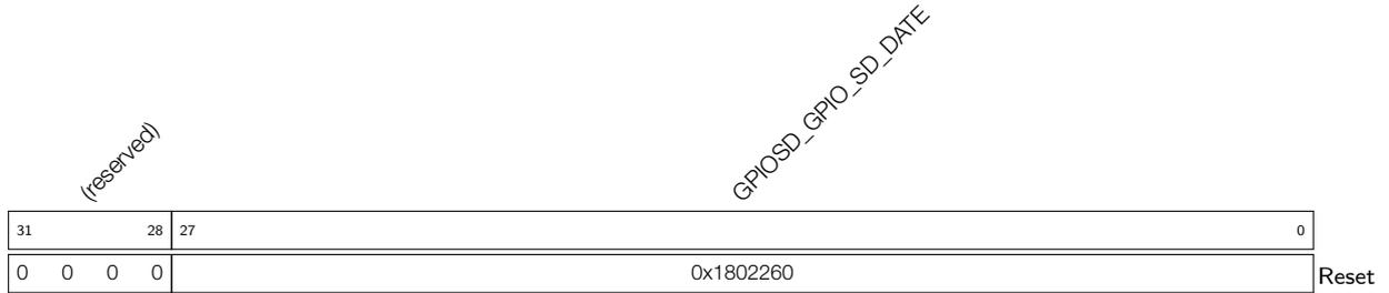
**GPIOSD\_GPIO\_SD\_DATE** Version control register. (R/W)
