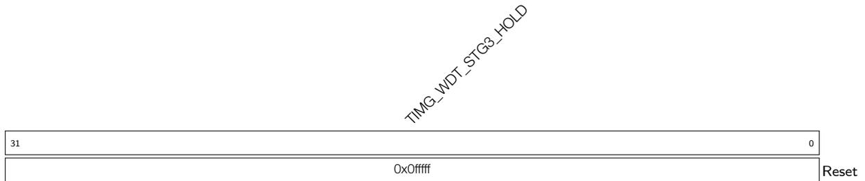
**TIMG\_WDT\_STG3\_HOLD** Stage 3 timeout value, in MWDT clock cycles. (R/W)
