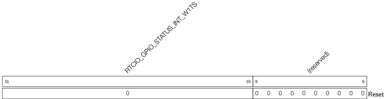
**RTCIO\_GPIO\_STATUS\_INT\_W1TS** GPIO0 ~ 21 interrupt set register. If the value 1 is written to a bit here, the corresponding bit in [RTCIO\\_GPIO\\_STATUS\\_INT](#) will be set to 1. Recommended operation: use this register to set [RTCIO\\_GPIO\\_STATUS\\_INT](#). (WO)
