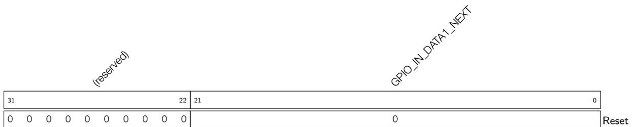
**GPIO\_IN\_DATA1\_NEXT** GPIO32 ~ 53 input value. Each bit represents a pad input value. (RO)
