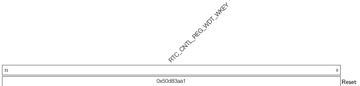
**RTC\_CNTL\_REG\_WDT\_WKEY** Sets the write protection key of the watchdog. (R/W)
