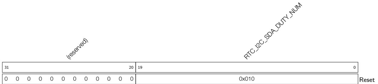
**RTC\_I2C\_SDA\_DUTY\_NUM** The number of clock cycles between the SDA switch and the falling edge of SCL. (R/W)
