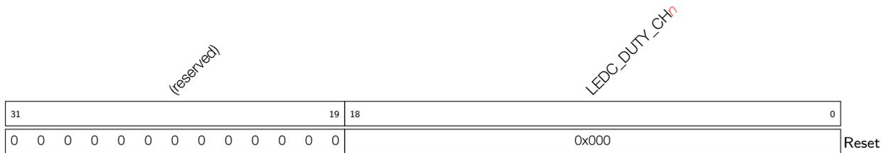
**LEDC\_DUTY\_CH $n$**  This register is used to change the output duty by controlling the Lpoint. The output value turns to low when the selected timers has reached the Lpoint. (R/W)
