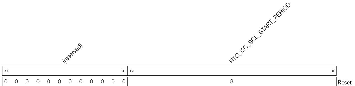
**RTC\_I2C\_SCL\_START\_PERIOD** Number of clock cycles to wait after generating a start condition. (R/W)
