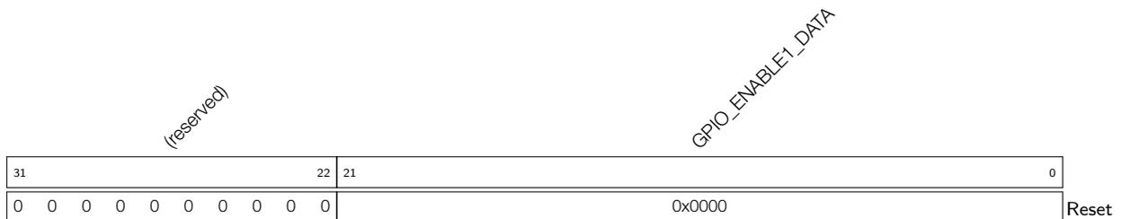
**GPIO\_ENABLE1\_DATA** GPIO32 ~ 53 output enable register. (R/W)
