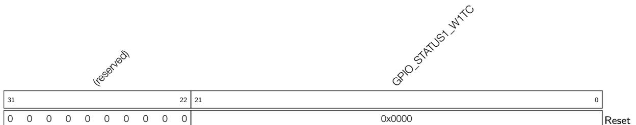
**GPIO\_STATUS1\_W1TC** GPIO32 ~ 53 interrupt status clear register. If the value 1 is written to a bit here, the corresponding bit in [GPIO\\_STATUS1\\_REG](#) will be cleared. Recommended operation: use this register to clear [GPIO\\_STATUS1\\_REG](#). (WO)
