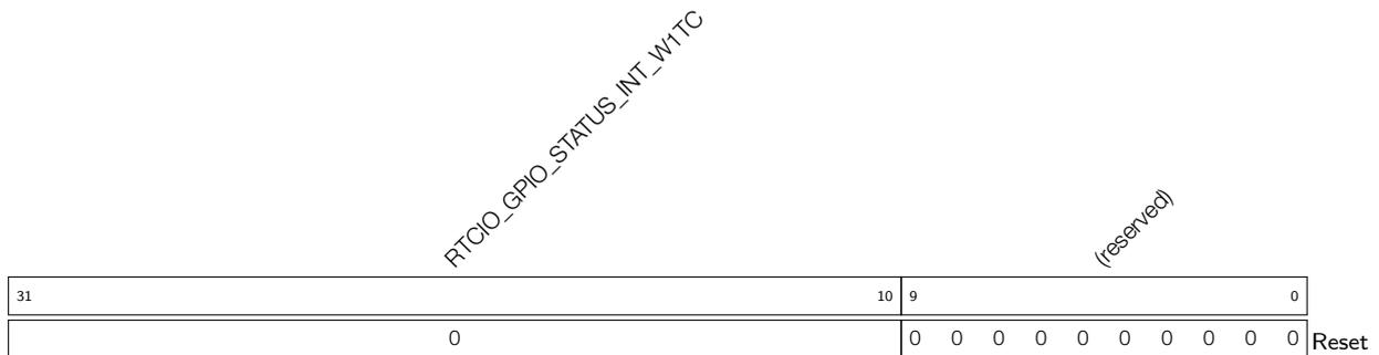
**RTCIO\_GPIO\_STATUS\_INT\_W1TC** GPIO0 ~ 21 interrupt clear register. If the value 1 is written to a bit here, the corresponding bit in [RTCIO\\_GPIO\\_STATUS\\_INT](#) will be cleared. Recommended operation: use this register to clear [RTCIO\\_GPIO\\_STATUS\\_INT](#). (WO)
