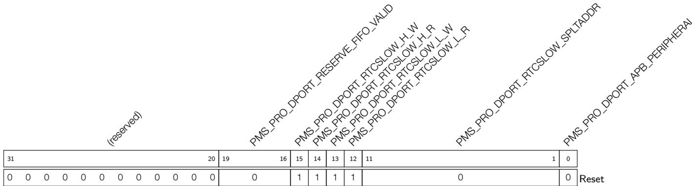
**PMS\_PRO\_DPORT\_APB\_PERIPHERAL\_FORBID** Setting to 1 denies PeriBus1 bus's access to APB peripheral. (R/W)
