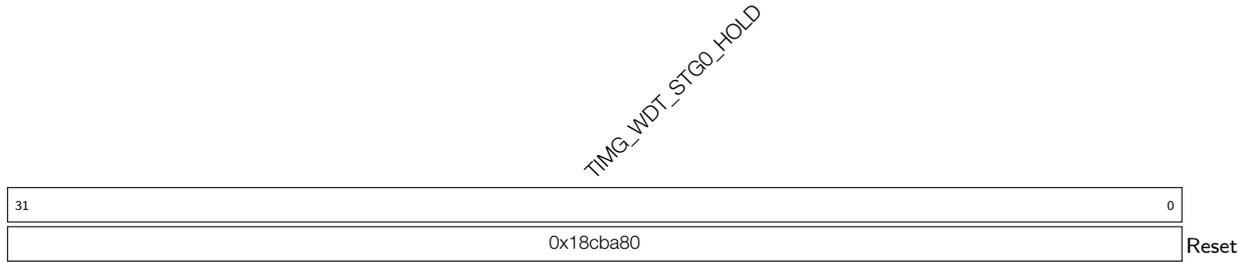
**TIMG\_WDT\_STG0\_HOLD** Stage 0 timeout value, in MWDT clock cycles. (R/W)
