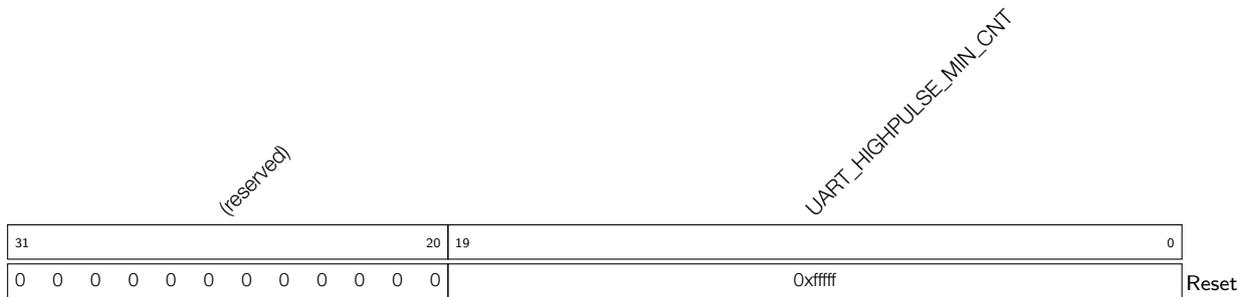
**UART\_HIGHPULSE\_MIN\_CNT** This register stores the value of the maximum duration time for the high level pulse. It is used in baud rate detection. (RO)
