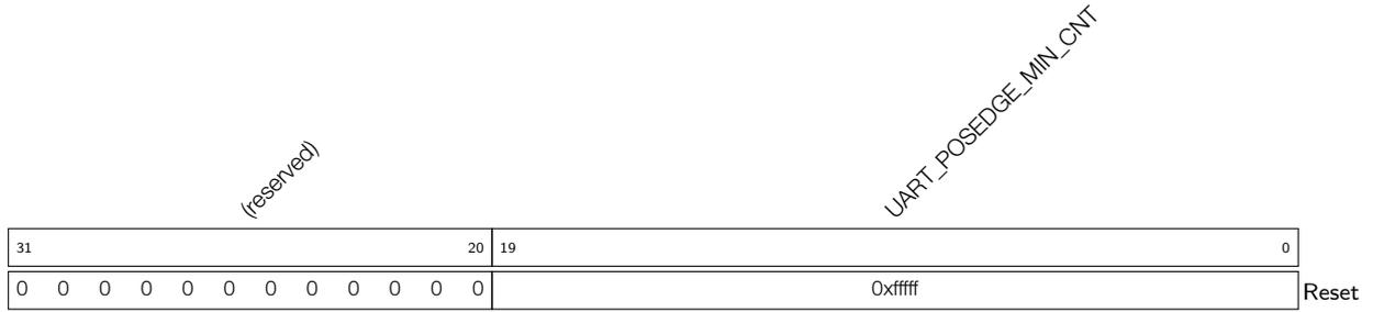
**UART\_POSEDGE\_MIN\_CNT** This register stores the minimal input clock count between two positive edges. It is used in baud rate detection. (RO)
