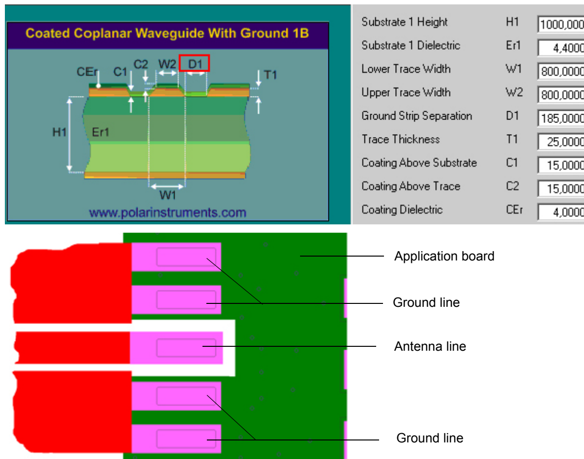
Figure 25: Micro-Stripline on 1.0mm standard FR4 2-layer PCB - example 1
