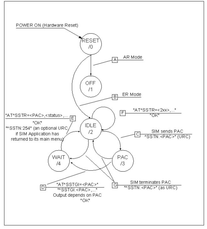
Figure 8.2: Remote-SAT State Transition Diagram
