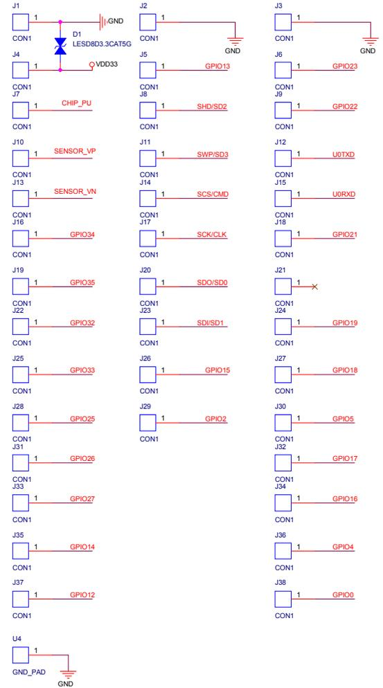
Figure 3: ESP32-SOLO-1 Schematics
