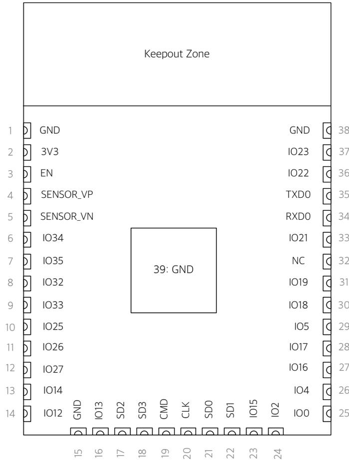
Figure 1: ESP32-SOLO-1 Pin layout
