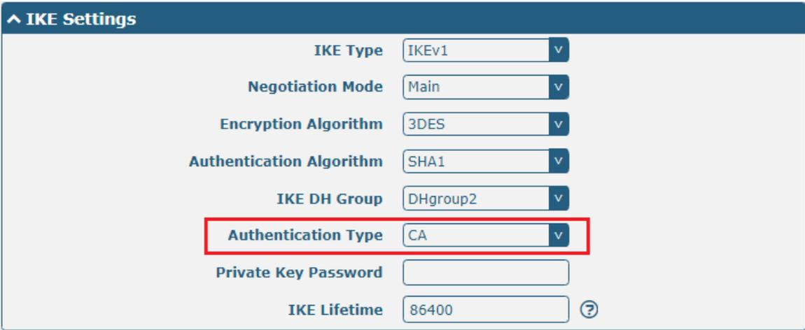
The screenshot shows the 'IKE Settings' configuration window. The 'Authentication Type' dropdown menu is highlighted with a red box and is set to 'CA'. Other settings include: IKE Type (IKEv1), Negotiation Mode (Main), Encryption Algorithm (3DES), Authentication Algorithm (SHA1), IKE DH Group (DHgroup2), Private Key Password (empty field), and IKE Lifetime (86400).
