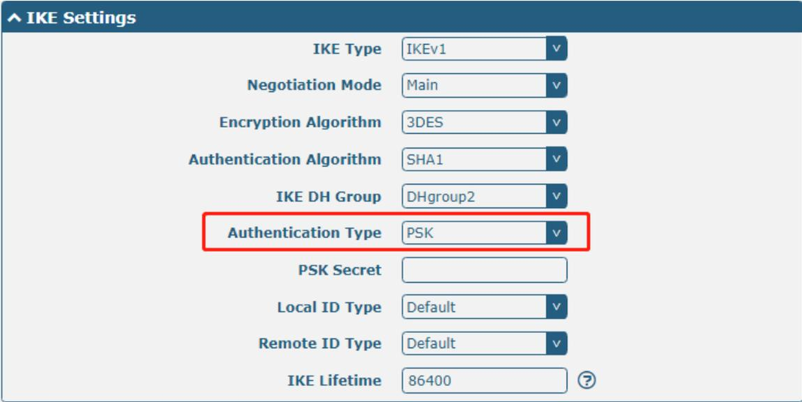
The screenshot shows the 'IKE Settings' configuration window. The 'Authentication Type' dropdown menu is highlighted with a red box and is set to 'PSK'. Other settings include: IKE Type (IKEv1), Negotiation Mode (Main), Encryption Algorithm (3DES), Authentication Algorithm (SHA1), IKE DH Group (DHgroup2), PSK Secret (empty field), Local ID Type (Default), Remote ID Type (Default), and IKE Lifetime (86400).
