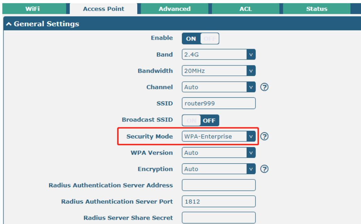
The screenshot shows the 'General Settings' for WiFi. The 'Security Mode' dropdown menu is highlighted with a red box and is set to 'WPA-Enterprise'. Other settings include: Enable (ON), Band (2.4G), Bandwidth (20MHz), Channel (Auto), SSID (router999), Broadcast SSID (OFF), WPA Version (Auto), Encryption (Auto), Radius Authentication Server Address (empty), Radius Authentication Server Port (1812), and Radius Server Share Secret (empty).
