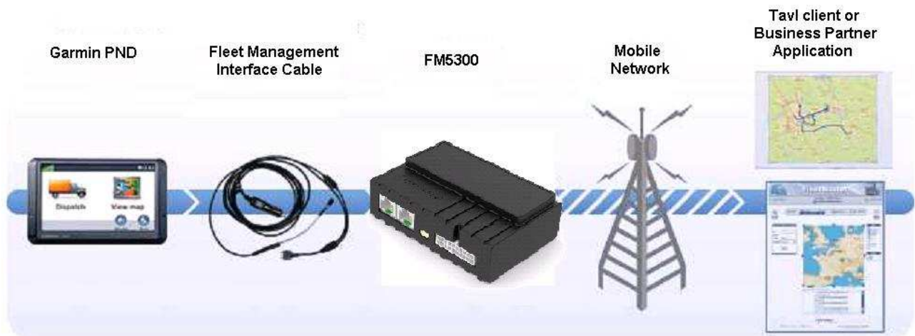
Figure 548 FM53+Garmin operational scheme
