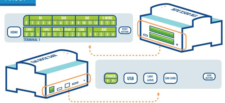
NPE X500 M3 - Industrial Embedded Computer based on the Linux system
