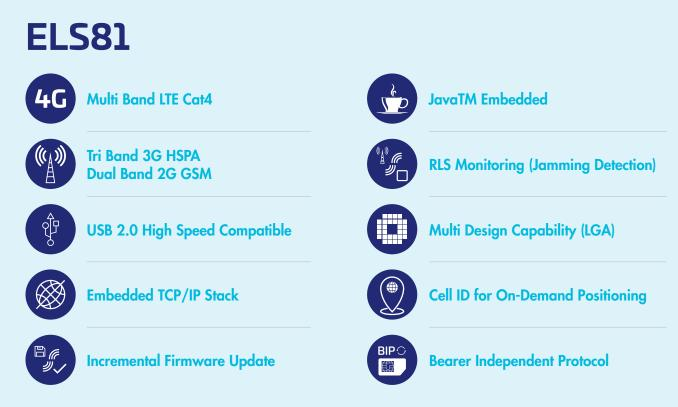
The Thales Cinterion® ELS81 IoT wireless module marries sizzling speed and high throughput with rugged IoT durability delivering Cat 4 LTE connectivity with seamless fall back to 2G and 3G networks. Enabling data speeds of 150 Mbit/s download and 50 Mbit/s uplink, the ELS81 IoT module is ideal for data intensive solutions such as digital signage, video security monitoring, advanced retail POS terminals and kiosks and tablets.
