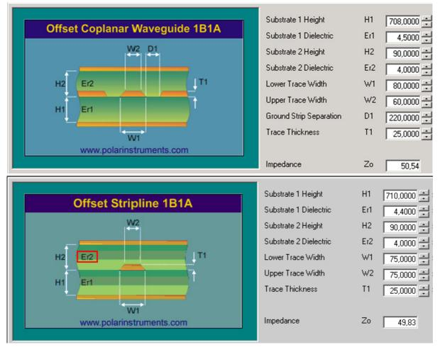
Figure 12: Embedded Stripline line arrangement
