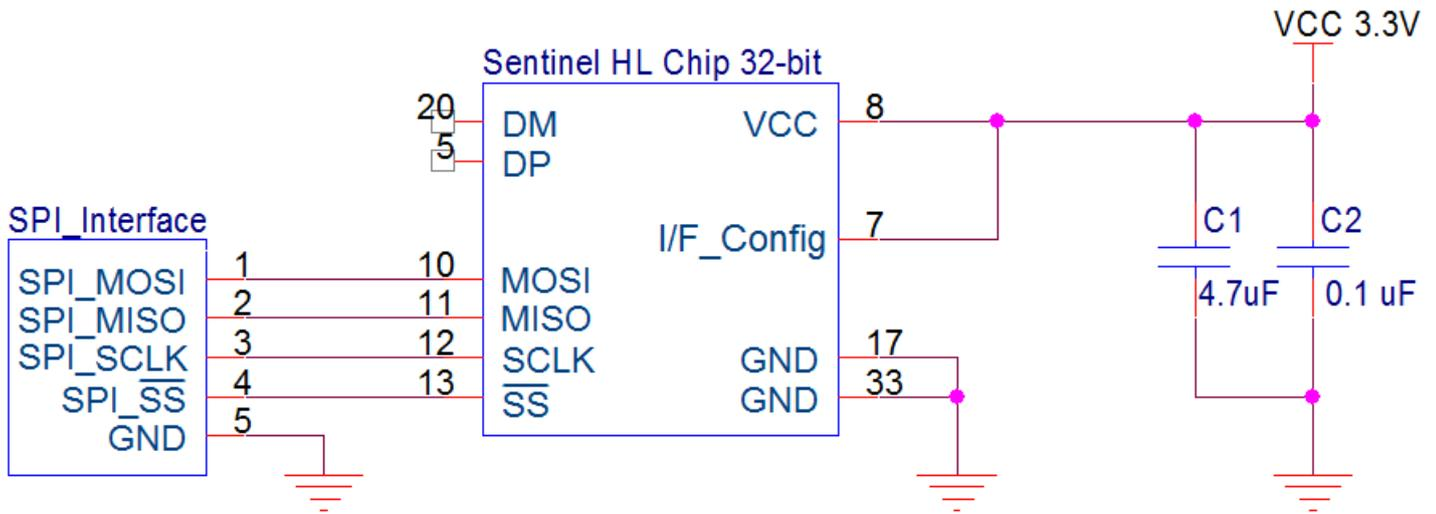
\* Pin 5 and Pin 20 can be left open in this application.
