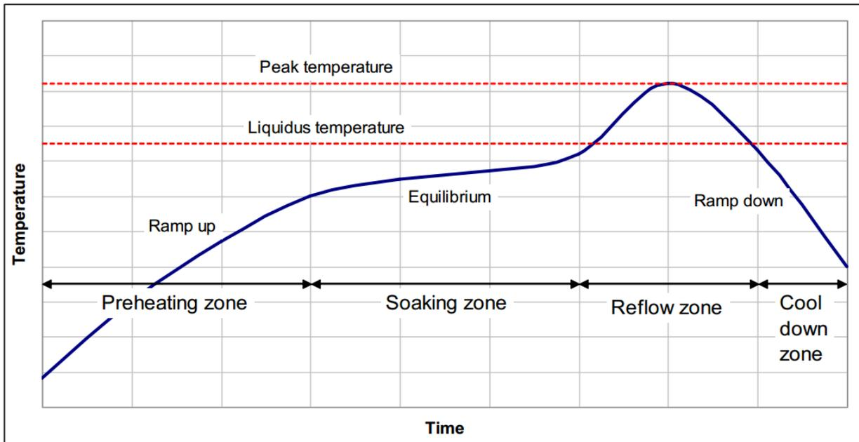
Example of the key data for a forced-convection reflow solder profile
