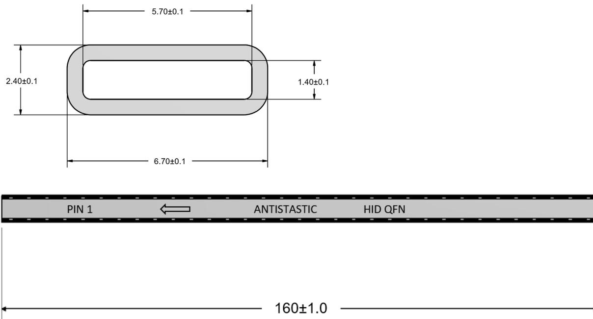
Figure 4: Tube 2 Dimensions (mm)
