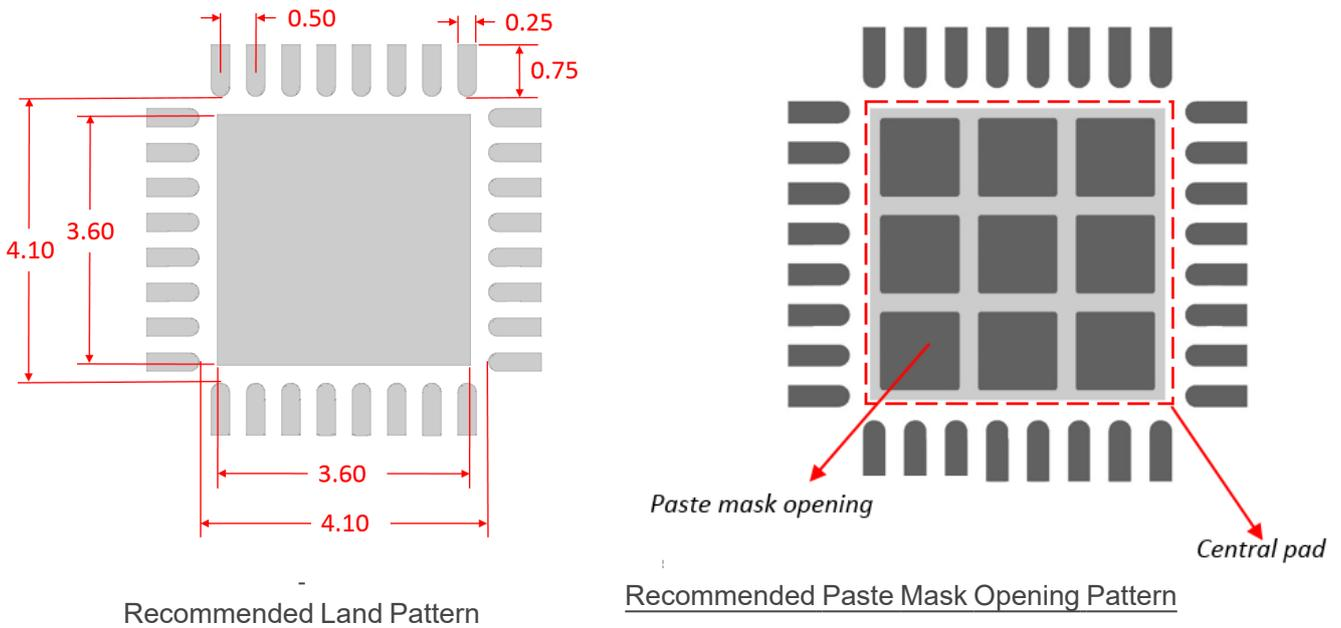
The area of paste mask openings should account for more than 60% of the whole area in the central pad.
