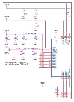
Figure 3: ESP32-S2 Analog Power Supply Pins
