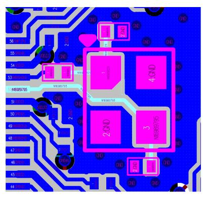
Figure 14: ESP32-S2 Crystal Oscillator Layout
