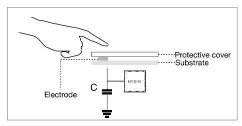
Figure 18: A Typical Touch Sensor Application
