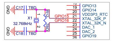
Figure 7: Schematic for ESP32-S2's External Crystal (RTC)
