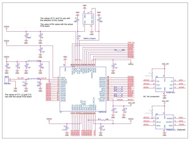
Figure 1: ESP32-S2 Schematic
