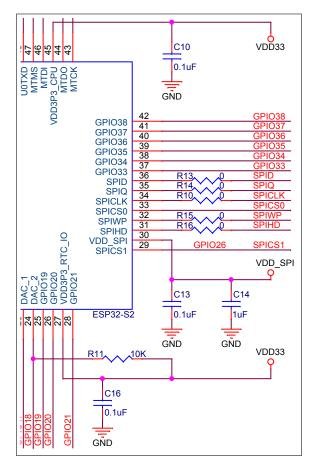
Figure 2: ESP32-S2 Digital Power Supply Pins
