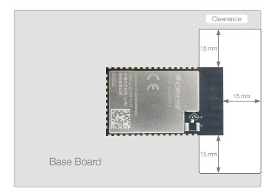
Figure 12: Keepout Zone for ESP32-S2 Module's Antenna on the Base Board
