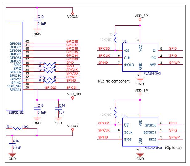
Figure 4: ESP32-S2 Flash and SRAM
