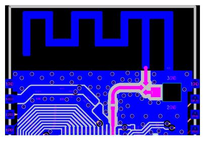
Figure 15: ESP32-S2 RF Layout in a Four-layer PCB Design
