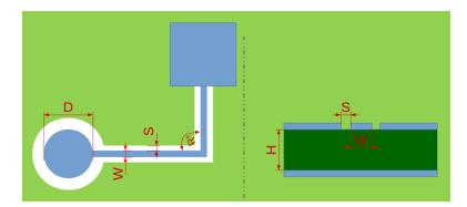
Figure 20: Sensor Track Routing Requirements
