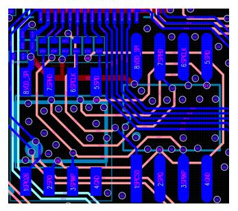
Figure 17: ESP32-S2 Flash and PSRAM Layout
