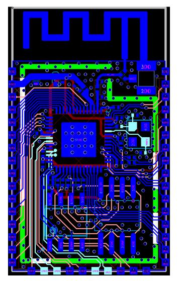
Figure 10: ESP32-S2 PCB Layout
