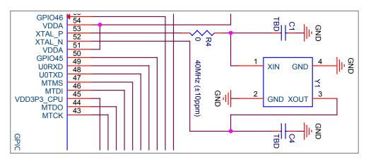
Figure 5: Schematic for ESP32-S2's Crystal
