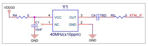
Figure 6: Schematic for ESP32-S2's Crystal Oscillator
